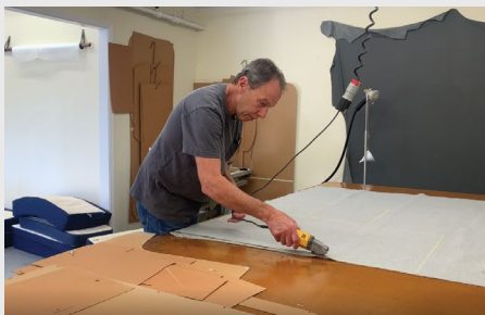
1. The fabric pattern (flatwork) for the chair seat cushion is cut out of the cover fabric laminated with the fire barrier.
