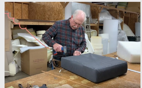
If installed separately, the barrier (shown in gray) must go under the cover fabric and fully encapsulate the foam.
