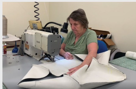
2. The flatwork for the seat cushion is assembled. Alternatively, the cover fabric and barrier can be stapled.
