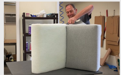
3. The cover fabric and fire barrier are installed at once, entirely encapsulating the foam cushion.
