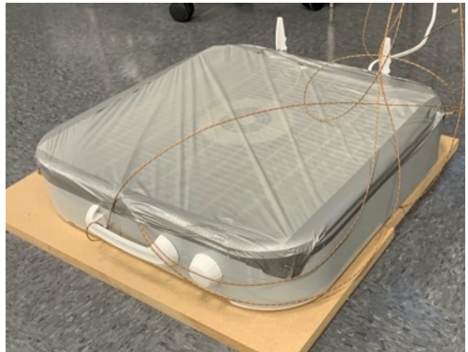
FIGURE 3. PICTURES OF THE TESTED BOX FANS WITH THERMOCOUPLES ATTACHED, ONE SIDE BLOCKED (LEFT) AND BOTH SIDE BLOCKED WHEN LYING FACE DOWN (RIGHT).
