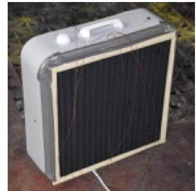
Fan with dust laden filter
